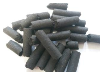
Fig. 2. General view of pellets produced from torrefied waste forest biomass.
