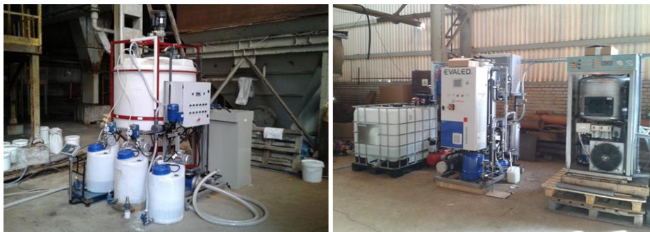
Fig. 1. Wastewater treatment pilot plant view (left – chemical neutralization unit, right – evaporation and crystallization unit).
