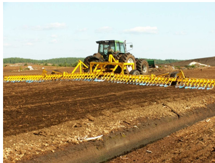
Fig. 3. Work process of a milled peat tedder on the drained peat deposit.
