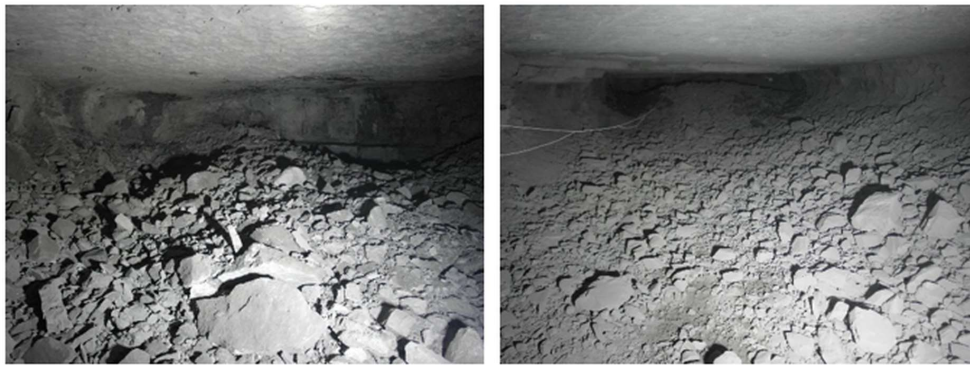
Fig. 6. View of the mining faces after blasting using regular drilling and firing pattern: face A (left) and face B (right).
