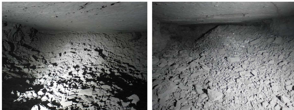
Fig. 7. View of the mining faces after blasting using modified drilling and firing pattern: face C (left) and face D (right).
