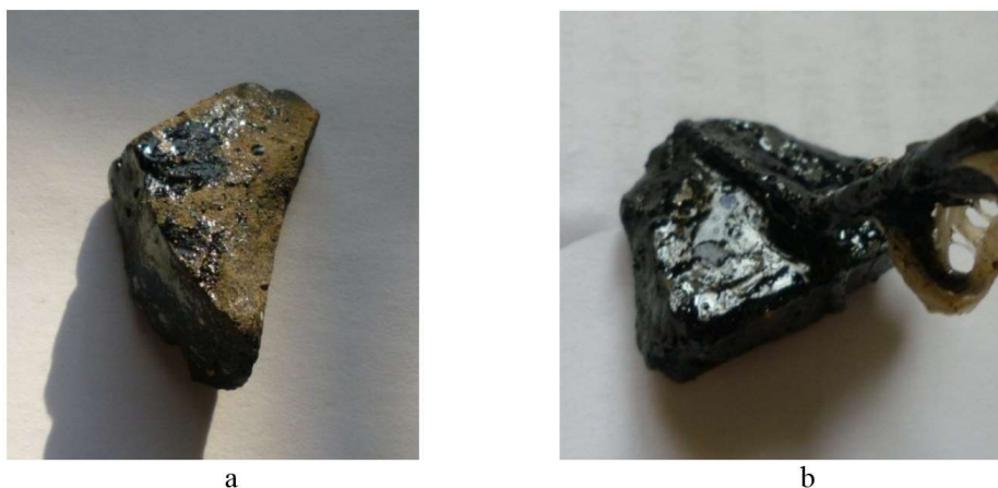
Fig. 1 Adhesion of: a) BND 60/90 bitumen and b) bitumen modified with crumb rubber by stages to 5-20 mm fraction Krapivinskiy quarry crushed stone.
