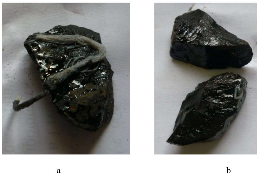
Fig. 2 Adhesion of bitumen modified with crumb rubber by stages to 5-10 mm fraction: a) Moszhukhinskiy and b) Gurievskiy quarries crushed stone.
