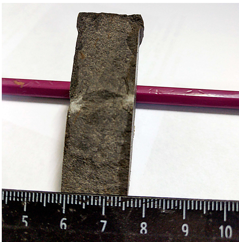
Fig. 4. The water-saturated sample of siltstone.
