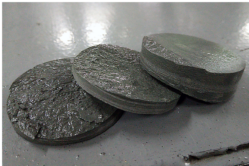
Fig. 5. Stratification of silt sample into 3 discs.
