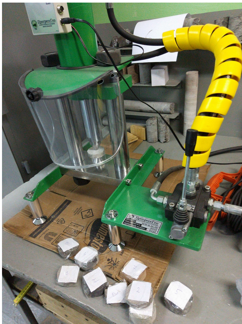
Fig. 1. The sample loading by PSN-0.16.10 lumped-loading device.
