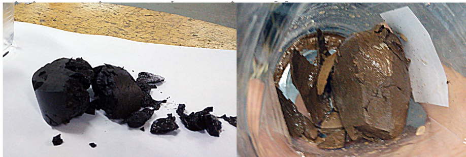
Fig. 3. The destroyed water-saturated samples of argillite (left) and marl (right).
