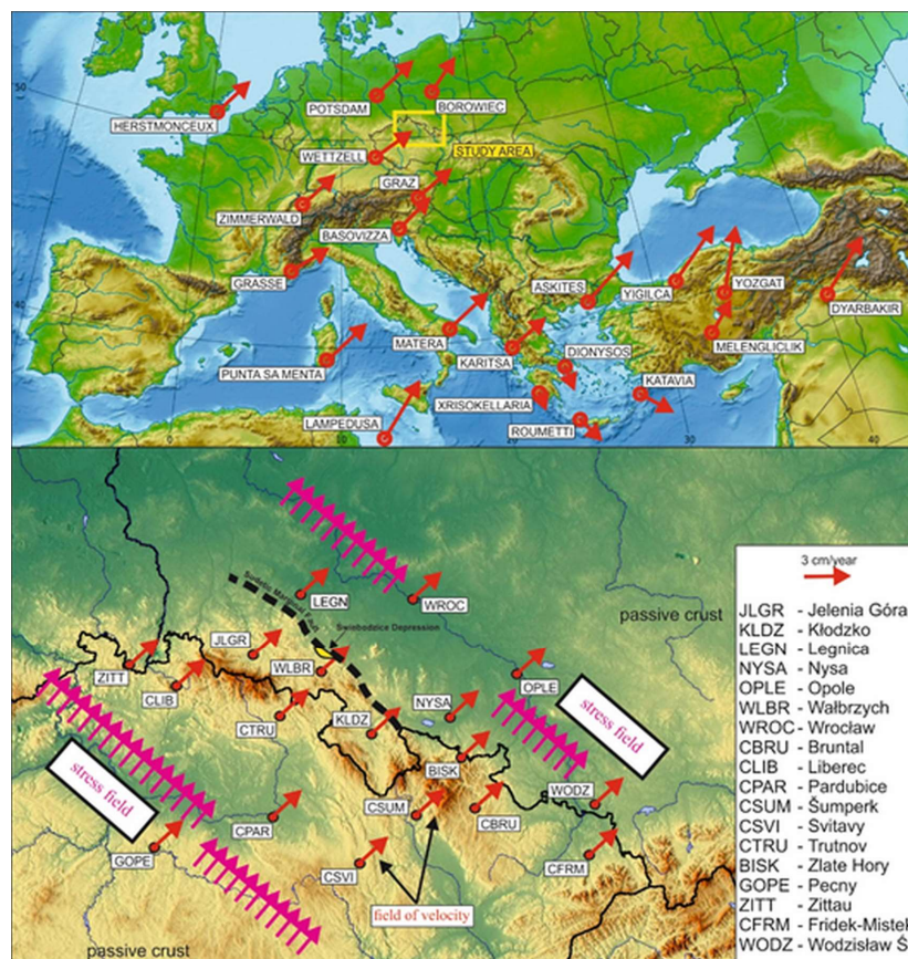
Fig. 1. Vectors of horizontal velocity plotted from GNSS data [33].
