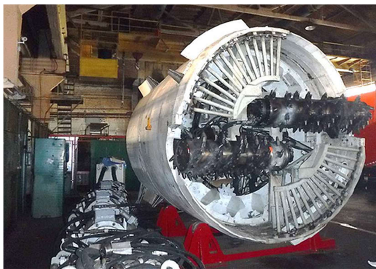
Fig. 2. Experimental sample of Geohod with drum-like working body.
