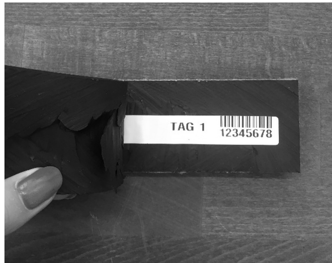
Fig. 2. Insertion of the tag into the test specimen.
