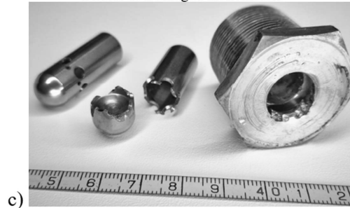
Photo 2. Damaged elements of valves
