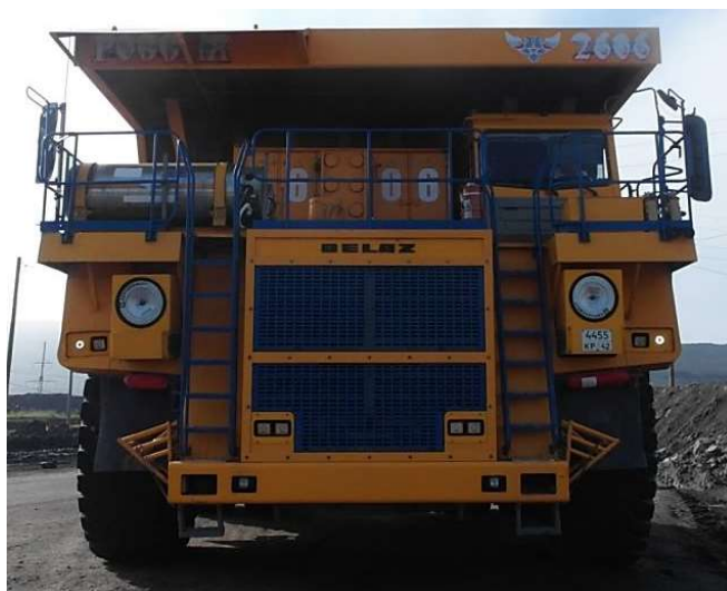
Fig. 3. High-payload-capacity BelAZ 75131 haul truck equipped with on-board cryogenic fuel system.
