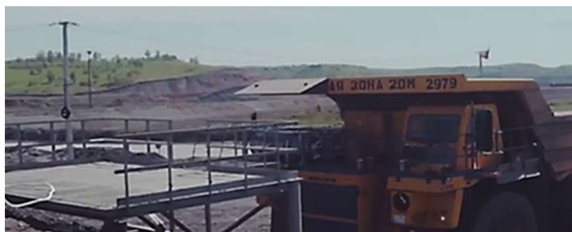
Fig. 2. Area for refueling haul trucks with liquefied natural gas.
