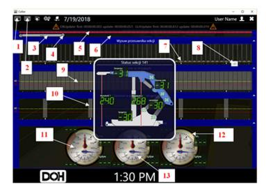
Fig. 2. Display of results of monitoring the work parameters of the powered roof support section.
