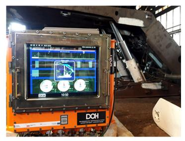
Fig. 4. Interface for monitoring the operation parameters of the longwall system during bench tests of the support section.
