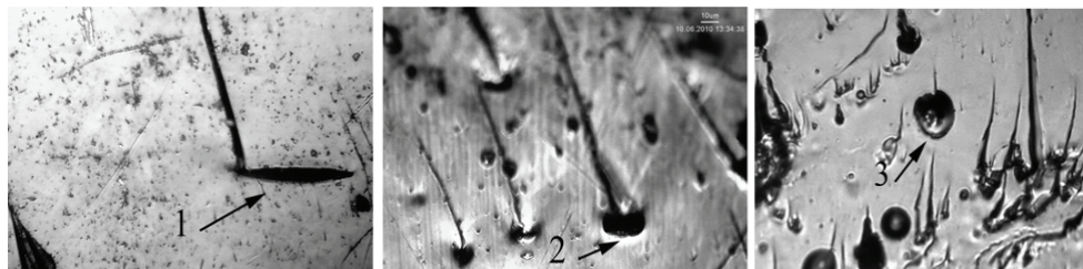
Fig. 4. Sequential (1, 2, 3) transformation of lenticular cavity into a sphere at the formation of a gas bubble.
