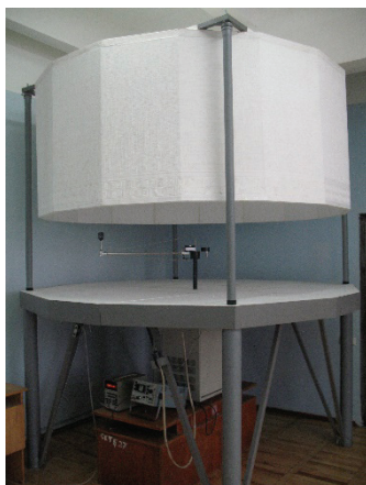
Fig. 1. Working standard of the speed of the air flow of the RESVP-1 in preparation for research of high-precision converter of an anemometer APR-2 of the third modification.
