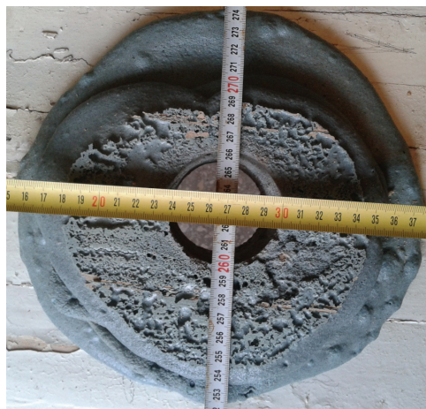
Fig. 4. Distribution radius of TCM in a crack with an opening of 30 mm.
