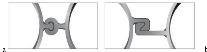
Fig. 15. Types of lock elements of pile wall technology: a - lock type WoM/WoF; b - lock type C6.
