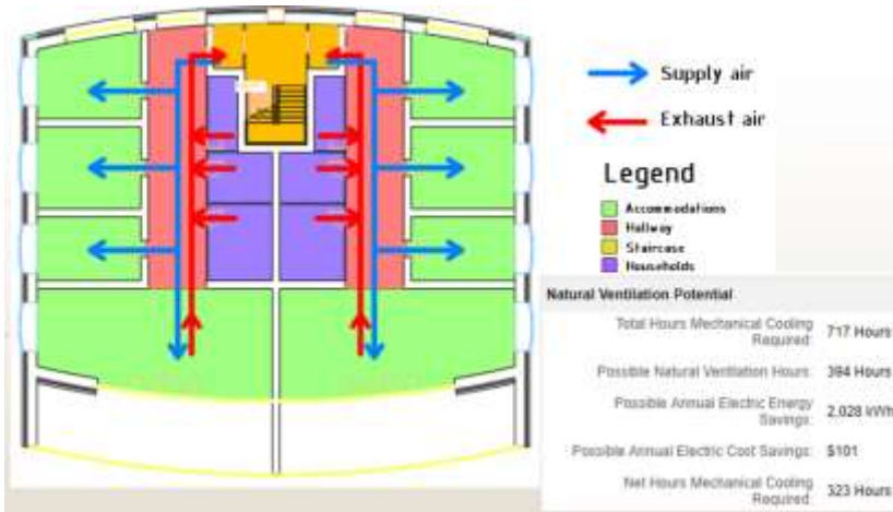
Fig. 5. Rational use of natural ventilation.
