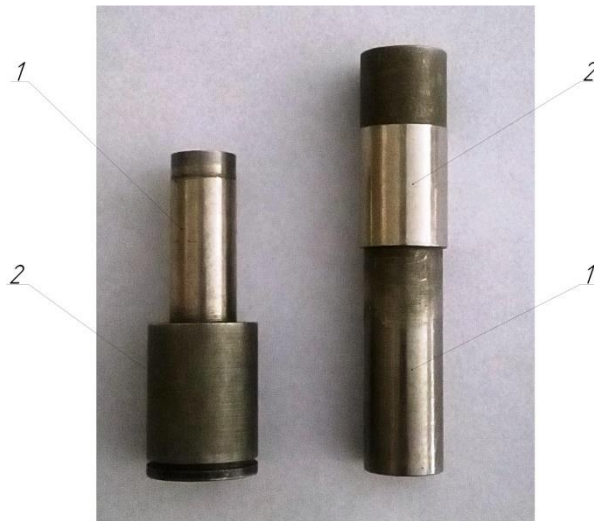
Fig. 6. Weldable cathode assemblies 1 – the core of the cathode; 2 – emitter
