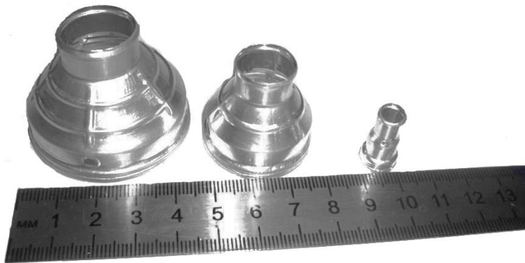
Fig. 2. Shielding housings of electric connectors of 3 standard sizes
