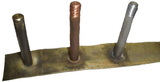
Fig. 4. Experimental sample: L63 sheet steel alloy, core elements from L63, M01 and AMg6 alloys
