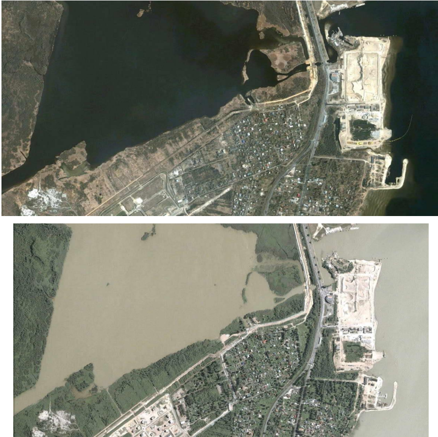
Fig. 2. Concentration of suspended material in the North Lakhta area before the construction of «Marine Facade of St. Petersburg» (above, 2004) and during the dredging work (below, 2011).
