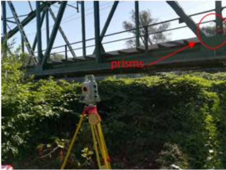
Fig 2. Used geodetic equipment Leica TS 50 and prisms.
