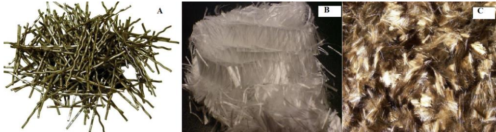
Fig. 1. Reinforcing fiber: A - steel; B - polypropylene; C – basalt.
