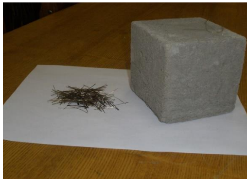
Fig. 4. Basalt fiber and foam fiber concrete block.
