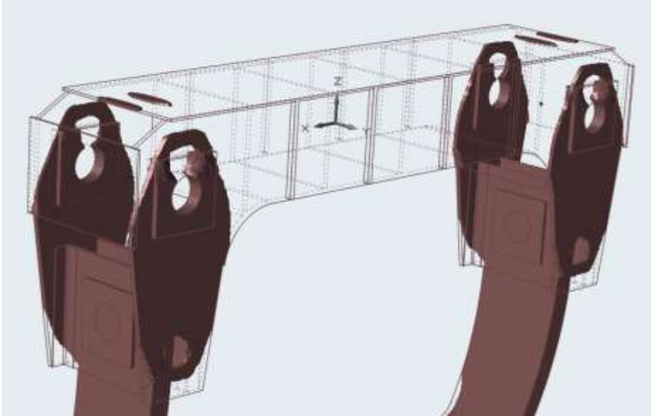
Fig 10. Traverse after design study using topological optimization method.
