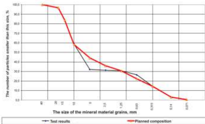
Fig. 10. The test results of the mixture at a temperature of +20°C (immediately after the preparation) B30 P3 F200 W2
