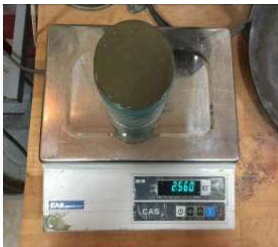
Fig. 4. The weighing of the selected sample to determine its density
