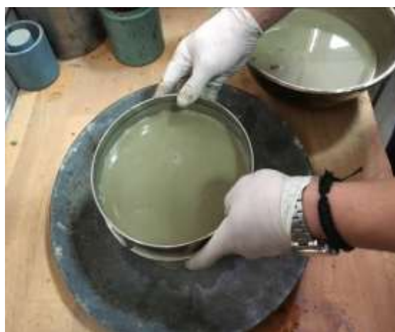
Fig. 5. Washing out the cement-concrete mixture
