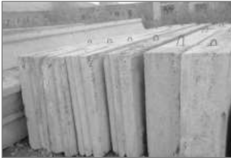
Fig. 3. Wall keramzit concrete panels.
