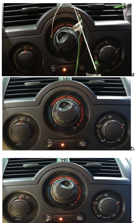
Fig. 5. Setup of the three position of the ventilation/climatization system a. V1, b. V2, c. V3
