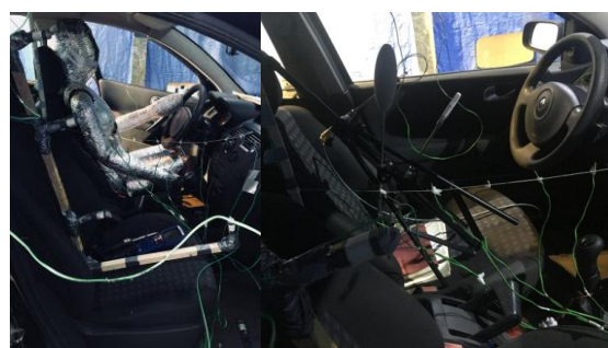
Fig. 4. Images during the experimental sessions with thermal manikin and CS
