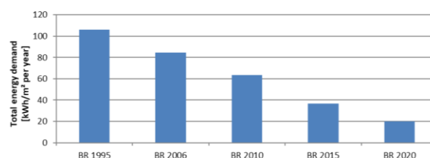
Fig. 1. The previous and new energy requirements for a new typical detached single-family house in Denmark. The requirements of BR2015 corresponds to the current BR2018 requirements.
