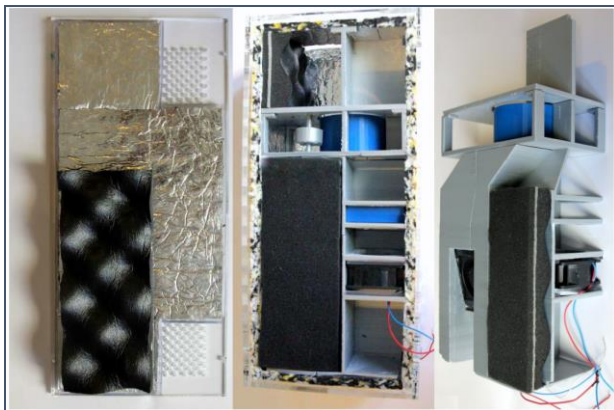
Fig. 4. Photos of the dehumidifier prototype in acrylic box with muffling material applied [5]
