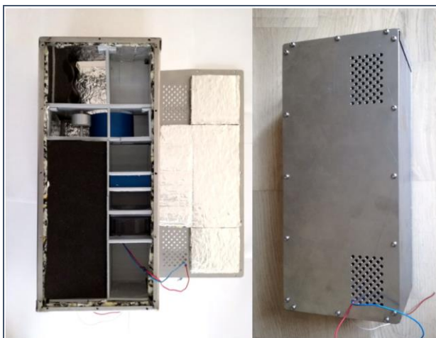
Fig. 5. Photos of the dehumidifier prototype in metal box [5]
