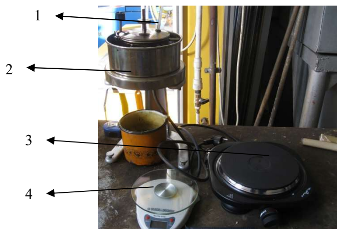
Fig.1. The equipment used to determine viscosity for animal fat mixed in liquid hydrocarbons
