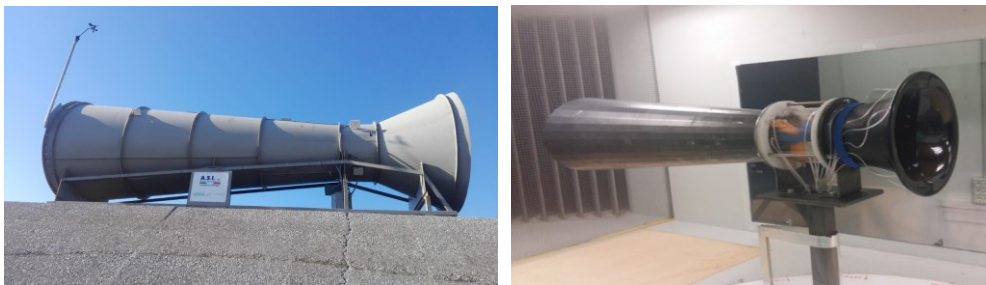
Fig. 1. Prototype of the wind ducted turbine installed in the harbour (left) and laboratory scale (right)
