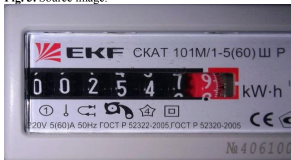
Fig. 4. Image with the elimination of perspective distortion.
