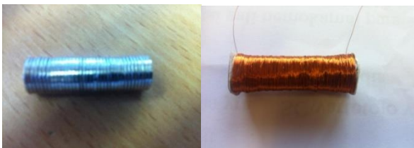
Fig.2. Micro electromagnetic generator and the Magnet used inside.
