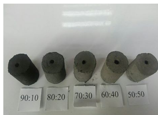
Fig 2. Physical characteristics of compressed bio-fuel made from Palm empty fruit bunches
