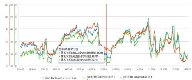
Fig.4. Inversion phenomenon of NO x monitoring result on a specific 600MW power unit
