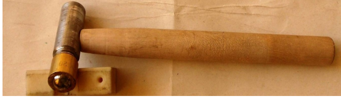
Fig. 3. The hammer with a spring-loaded spherical block head.
