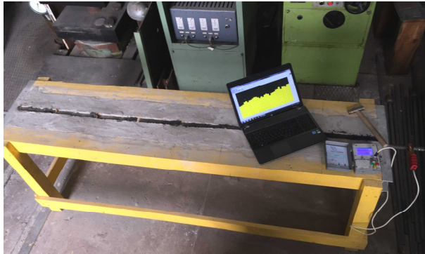
Fig. 2. Second test bench with the pre-tensioned rock bolt.
