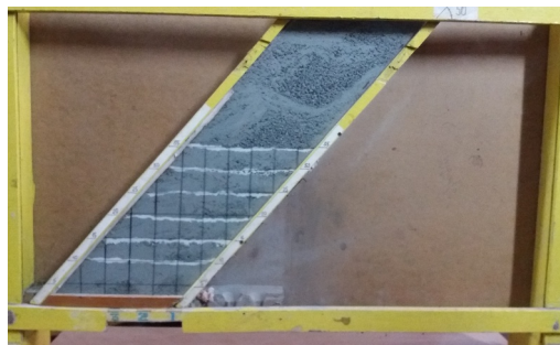
Fig. 2. The laboratory model for studying muck drawing.
