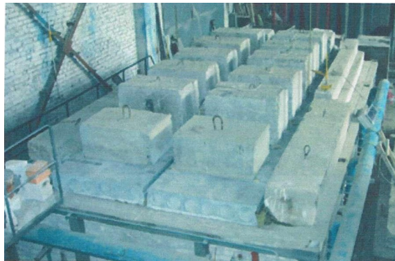
Fig. 9. Overall view of the floor slab samples before testing.
