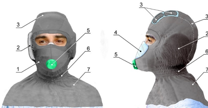
Fig. 1. CIPD of fast adjustment: 1 – balaclava; 2 – noise-attenuating elements; 3 – thermal accumulating elements; 4 – filtering gas and dust half-masks; 5 – valve unit; 6 – collar; 7 – cape [11].
