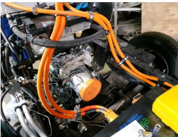
Fig. 4. Electric platform with gasoline generator.
