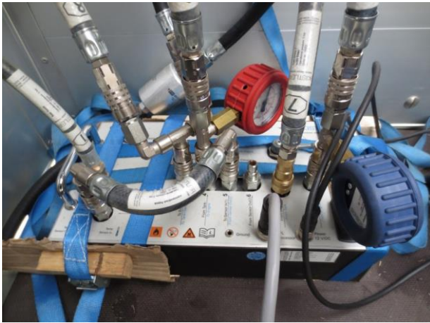
Fig. 5. Corrsys-Datron DFL3x fuel flow meter on GAZelle NEXT board with gasoline generator.
