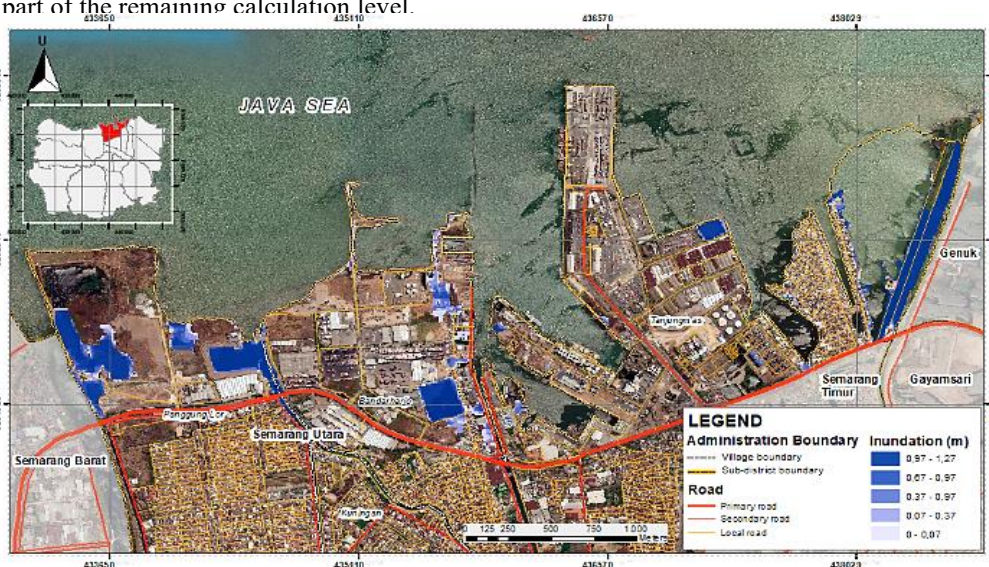
Fig. 7. Map of Tidal Flood Height in North Semarang Sub-District (Source: Analysis Results, 2019)
