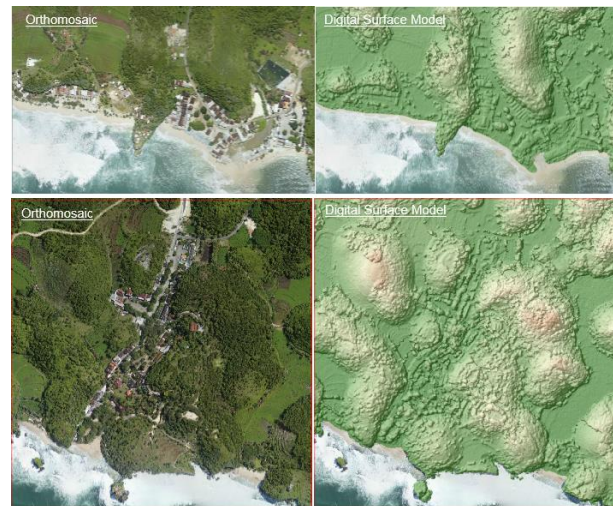
Fig. 2. Pieces of Orthomosaic (left) and DSM (right) of Watukodok-Drini Beach and Kukup Beach
