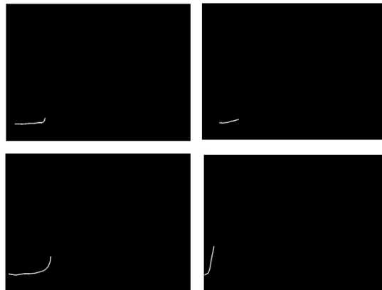
Fig. 9. Examples of black-and-white masks of reflection trace of E layer.
