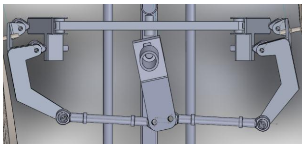
Fig. 5. Steering system using regular tie-rods.
