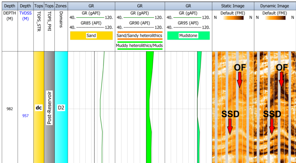
Fig. 4. Static and dynamic borehole electrical images, 981.5–982.5 m interval: example of open/conductive fractures (OF) and soft sediment deformation (SSD).
