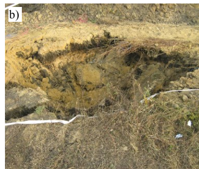
Photo. 3. Examples of sinkholes registered after de-stress blasting in the mining area of Piekary highway junction – a) and b) typical sinkholes for shallow cavities [5].
