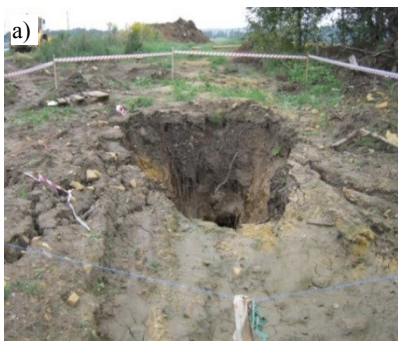
Photo. 3. Examples of sinkholes registered after de-stress blasting in the mining area of Piekary highway junction – a) and b) typical sinkholes for shallow cavities [5].
