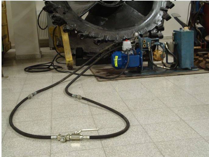
Fig. 4. Adjusting the settings of a hydraulic drive for supplying stand [2]
