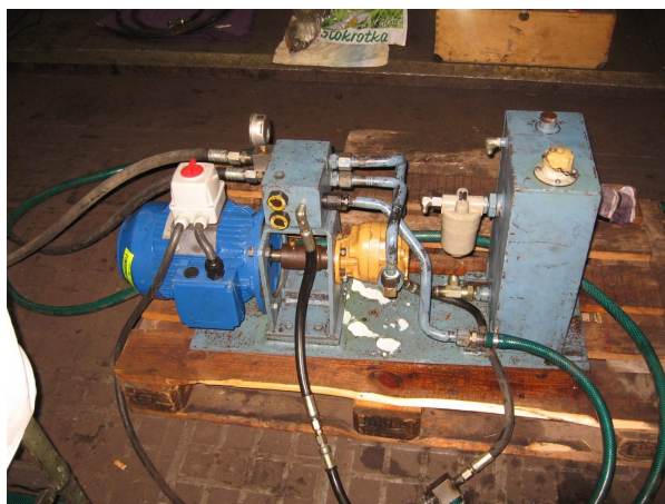
Fig. 5. Hydraulic drive on the test bench in HSW Stalowa Wola [2]
