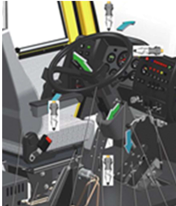
Fig. 1 The scheme of vibration measurement on the driver's seat, driver's cab, and steering wheel
