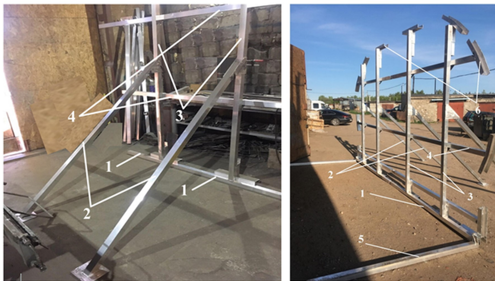
Fig. 5. The Appearance of the New Type of MVW Power Frame Assembled: 1 – base; 2 – supports; 3 – vertical racks; 4 – horizontal racks; 5 – skiing; 6 – groove.
