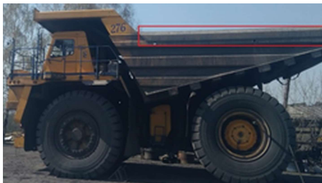
Fig. 1. BelAZ-7513 dump truck with extended side sides of the cargo platform.
