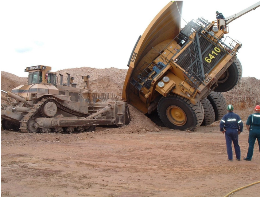
Fig. 1. A dump truck bogged down when unloading.
