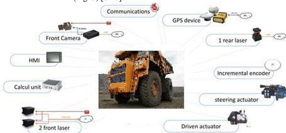
Fig. 3. Minimum equipment required for automated truck traveling.
