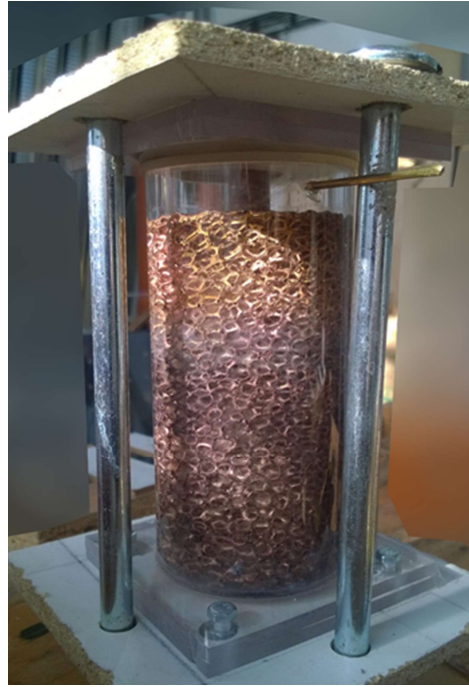
Fig. 5. Prototype of heat-storage unit based on PCM.
